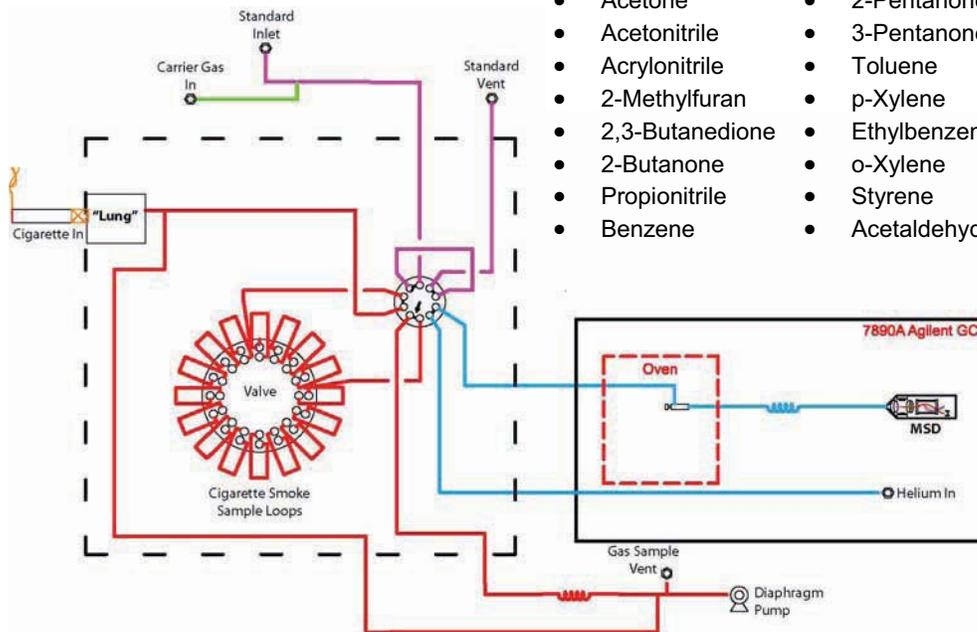
Figure 1: The plumbing diagram shows the Wasson-ECE cigarette puffing machine.
