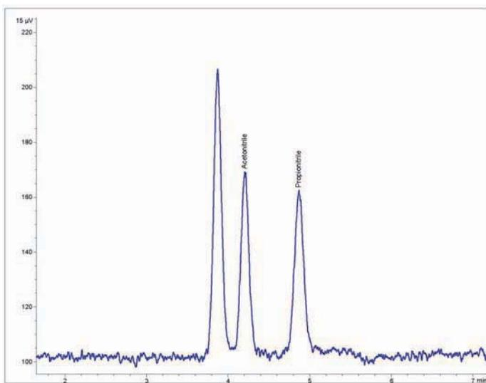
Figure 2: 2.5 µL liquid injection of 100 ppb acetonitrile and 100 ppb propionitrile diluted in MTBE
