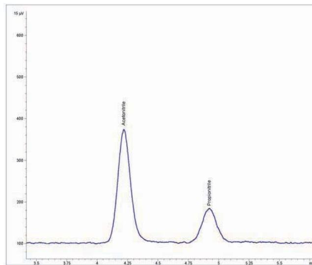
Figure 3: 2.5 µL liquid injection of 333 ppb acetonitrile and 333 ppb propionitrile diluted in TAME
